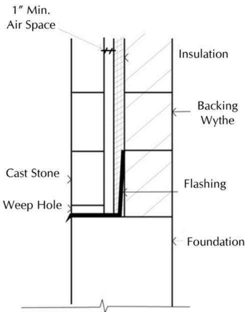
**DETAIL 1: Flashing at Base**
